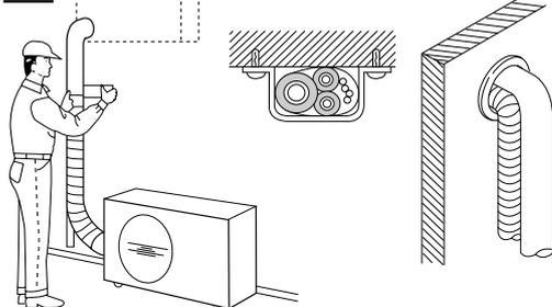
**EG** Complete insulation of refrigerant tubes; wrap with armoning tape. Fix and support tubes with brackets. Seal hole in the wall, if necessary.
