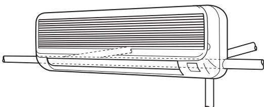
**EG** The unit can be connected to five directions: right rear - left rear - right side - left side and right downward.
