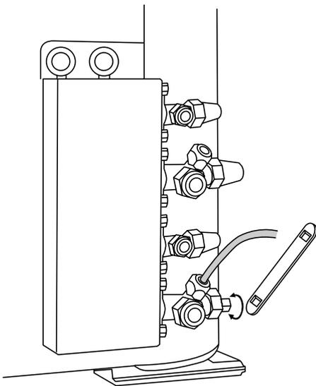
**EG** Turn the service valves stem in counterclockwise to fully open the valves. At this point vacuum pump flexible hose can be disconnected. Replace bonnet and flare nut, tighten them to 200 kg/cm with a torque wrench. Repeat what described from K to N for the second circuit. The two indoor units have to be marked has "indoor unit A" and "indoor unit B". Be sure that the idraulic connection to indoor unit A or B corrisponde to its own electrical connection.
