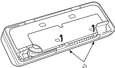
**EG** Press the 2  $\Delta$  marks on the frame cover and disengage the stationary tabs from the frame.
