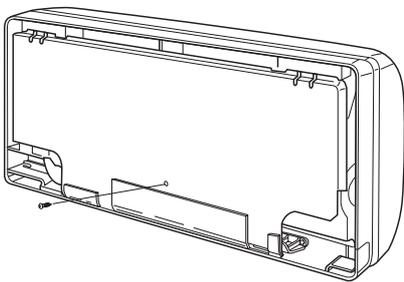
**EG** Remove and discard the set screw on the rear panel.
