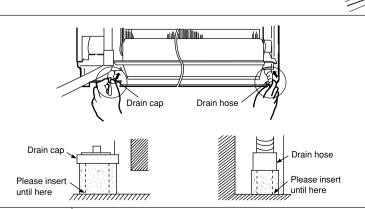
**⚠** CAUTION Condensed water may leak out if not inserted properly.
