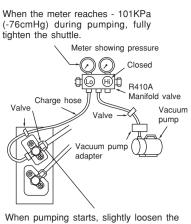
When pumping starts, slightly loosen the flare nut to check of air sucked in. Then
