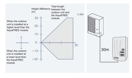
Maximum length of refrigerant piping Actual piping length  $\leq$  30 m Equivalent piping length  $\leq$  40 m
