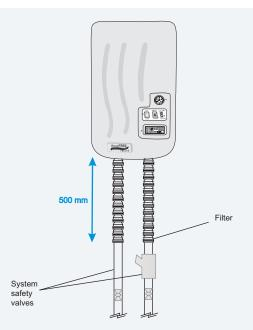
3. It is recommended to install a filter at the water inlet piping.
