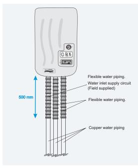
2. Install two valves. One at the water inlet pipe, and other at the water outlet pipe.
