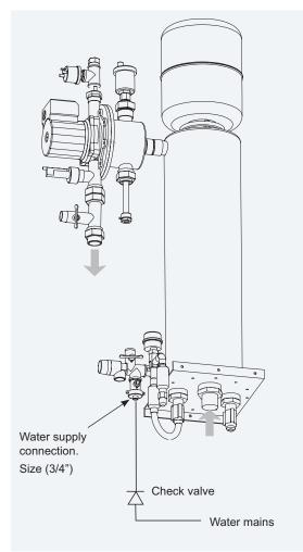
Charge the system with water by introducing it through the filling valve. The nominal pressure of the water of the system must be (1.7~2.0) bar. (Recommended 1.8 bar).
