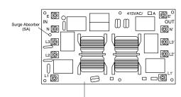
When the unit is applied the excessive surge current due to lighting or other causes, it is indicated this alarm code "04" or the inverter stoppage code (ITC) "11" and the unit can not be operated. In this case, check to ensure the surge absorber (SA) on the noise filter (NF1). If the inside of the surge absorber is normal, turn OFF the power once and wait for PCB2's LED OFF and turn ON again.
