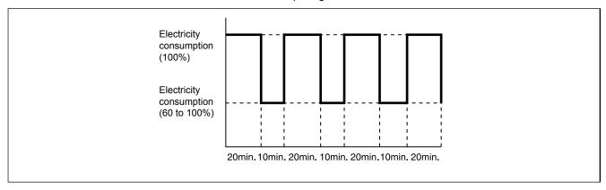
\* Wave function can be activated when demand function is selected at one of the input terminal indications if, in and if.
