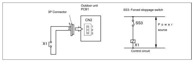
Wiring diagram example of demand current control
