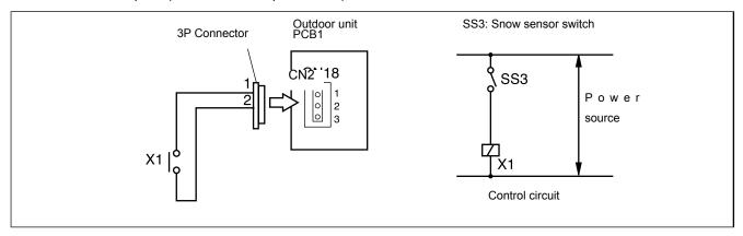
Wiring diagram example of snow sensor
