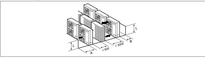
Keep a distance of more than 100mm between other units and do not put obstacles on the right and left sides. Dimension B is as shown beside.
