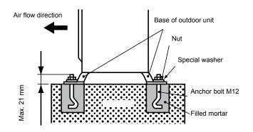
When installing the outdoor unit, fix the unit by anchor bolts. Refer to figure regarding the location of fixing holes.
