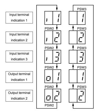
3 After the input/output terminal indication is selected, select your required control function No. by pushing PSW2 or PSW3 while PSW1 is being pushed.
