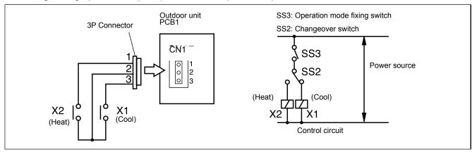
Wiring diagram example of fixing operation mode
