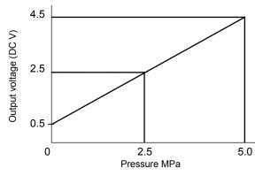
Output characteristics of high pressure sensor
