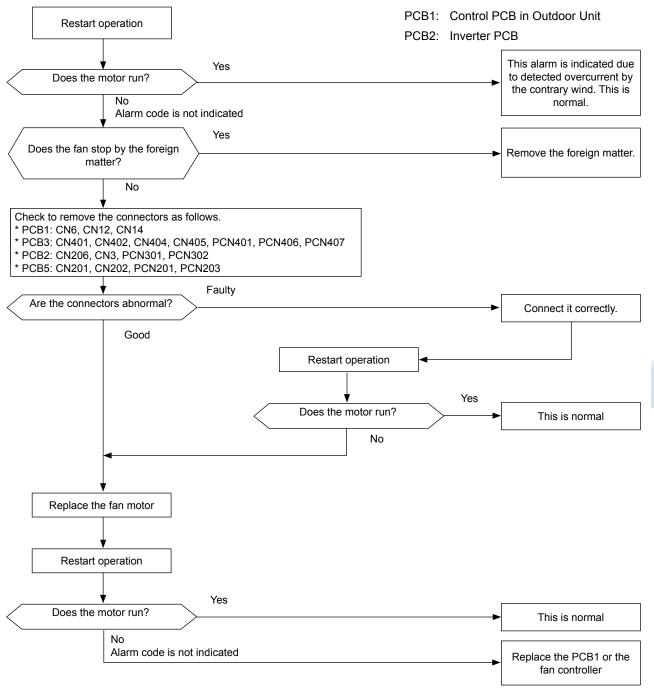
In the case that the fan motor does not run even the PCB1 is replaced, replace the PCB2
