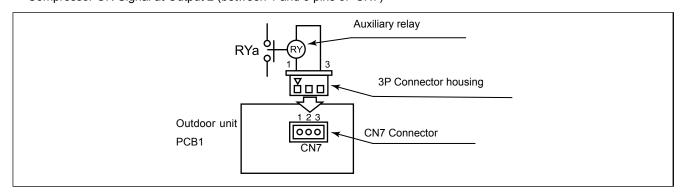
Wiring diagram example of compressor ON signal
