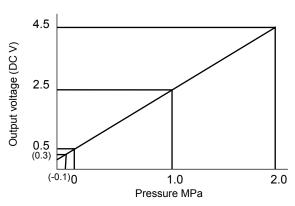
Output characteristics of low pressure sensor
