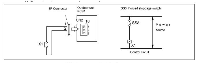
Wiring diagram example of forced stoppage
