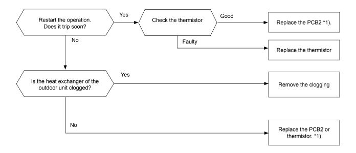
1\*): Refer to section "Procedure of checking other main parts" for the replacing procedure and the checking procedure for the PCB2.
