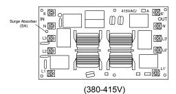
When the unit is applied the excessive surge current due to lighting or other causes, it is indicated this alarm code "04" or the inverter stoppage code (ITC) "11" and the unit can not be operated. In this case, check to ensure the surge absorber (SA) on the noise filter (NF1). If the inside of the surge absorber is normal, turn OFF the power once and wait for PCB2's LED OFF and turn ON again.
