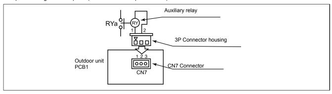
Wiring diagram example of operation signal
