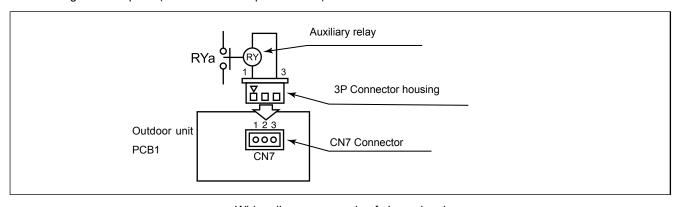
Wiring diagram example of alarm signal
