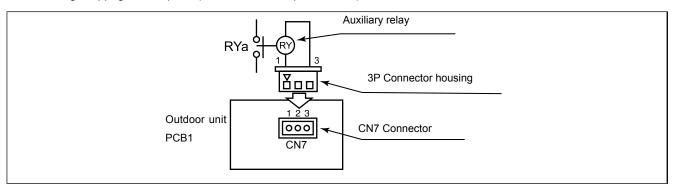
Wiring diagram example of defrosting signal
