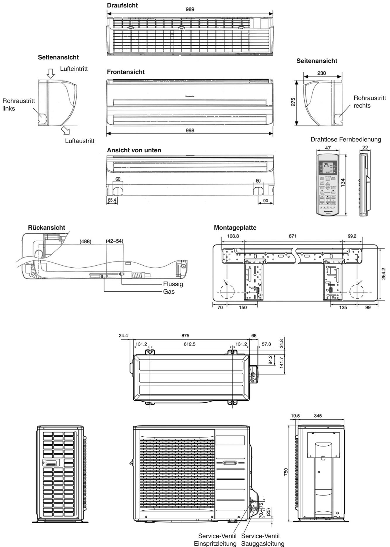
Abmessungen in mm
