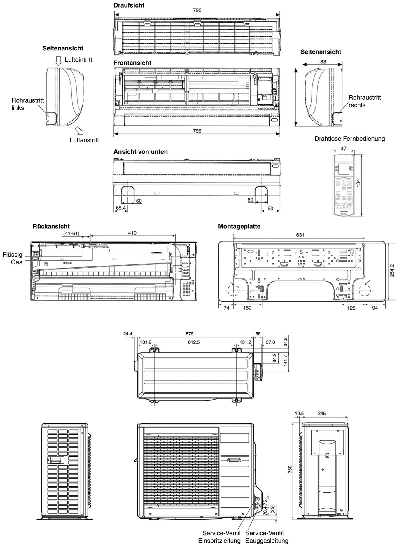
Abmessungen in mm
