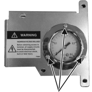
③ Remove 3 screws to remove pressure gauge.
