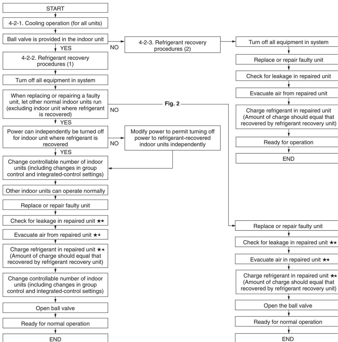
★ Service work performed on indoor units is done simultaneously using the service ports at the liquid (narrow tube) side and the gas (wide tube) side ball valves. Refer to each section in the "Installation Instructions" on refrigerant charging, leak checking, and evacuation procedures.
