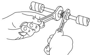
**EG** Tighten connections using a spanner and a torque wrench; apply specified torque (see table).
