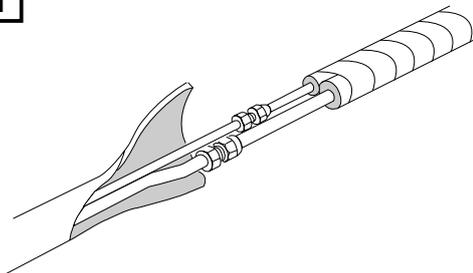
**EG** Insulate tubes leaving connections uncovered for leak test.
