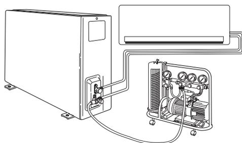
**EG** Air purging of internal unit and refrigerant tubes. Connect the vacuum pump to the outside unit as shown in the figure. Air and moisture have undesirable effects on the refrigerant system.
