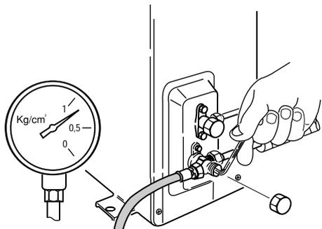
**EG** Turn on the unit's operating switch and start cooling operation. When the low-pressure gauge reading falls to 1 to 0,5 kg/cm<sup>2</sup>, fully close the wide tube stern and then quickly turn off the unit.
