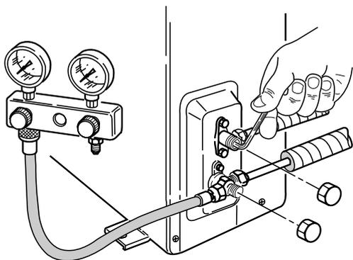
**EG** Connect a valve manifold to the charge port on the wide tube service valve, partially open it (1/4 turn). Let the air purge from the manifold. Fully close the narrow tube service valve all the way.
