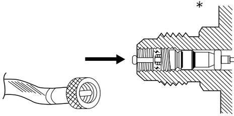
**EG** The service port on the wide tube service valve uses a Schrader core valve to access the refrigerant system. Therefore, be sure to use a hose connector which has a push-pin inside.
