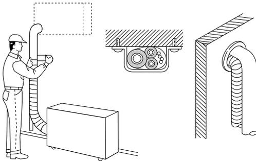
**EG** Complete insulation of refrigerant tubes; wrap with insulation tape. Fix and support tubes with brackets. Seal hole in the wall, if necessary.
