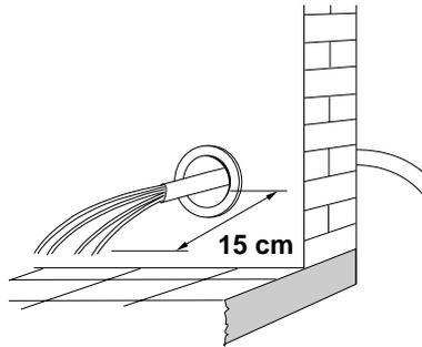
**EG** Make the holes for the fixing of the unit. Running power electric cable (with a ground wire) between the two units (see the table of wire section). Check if the quantity and the rawl plugs type supplied are the proper ones for fixing the unit on the wall.
