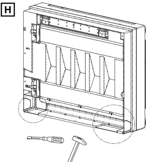
**EG** Open a pre-punched hole for the pipe passage (work from outside).
