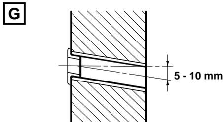
**EG** Drill a hole (see table), insert a PVC pipe.
