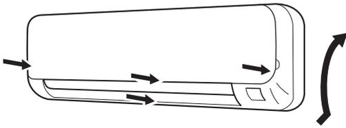
**EG** To fix the front panel again, insert it in the lower side of the unit and align it with the blocking points. Then push lightly on the shown marks.
