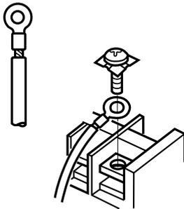
**EG** Predispose the terminals of the wire to connect to the terminal strip, connect them and secure the wiring with clamp provided. (See wiring diagrams).
