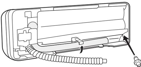
**EG** The refrigerant tubes and drain hose are on the right side of the unit.
