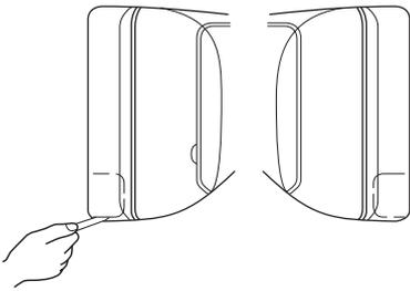
**EG** Tubing connections on right or left side. Cut a corner of the frame.
