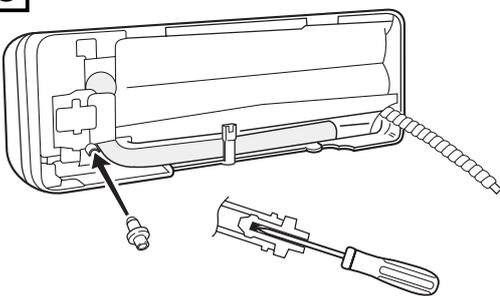
**EG** How to reverse the drain hose position. Remove the drain hose by turning it counterclockwise, then remove the rubber plug on the other side of the unit. Replace them inverting their position, use a screwdriver to place the plug correctly.
