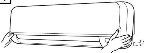
**EG** Push lightly to fix the unit to the rear panel.
