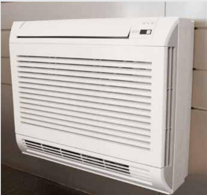
AF is equipped with DCM (DC motors) and is fitted with a humidity sensor used to modulate the temperature according to the temperature index perceived or to limit the maximum percentage of relative humidity in the environment. In addition, as shown in the figure, the two fans are activated in a differential mode to provide the best air distribution according to the operating cooling or heating mode.
