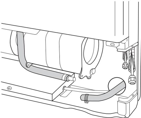
**EG** Predispose the condensate drain pipe and attach it to the fan housing if necessary.
