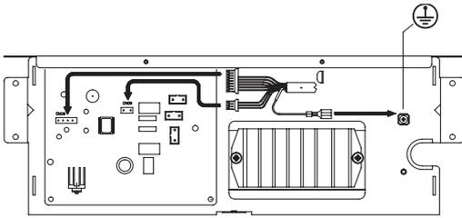
**EG** Perform the earth connection with the terminal on the base, as provided. Complete earth connection and fasten the other end of the cable to the earth terminal in the electric panel.
