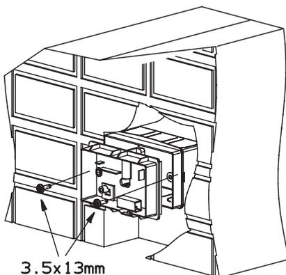
**EG** If allowed by the local electric-power standards, standard electric-component boxes can be used for assembling the receiver.
