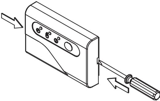
**EG** Slot a screwdriver by the 2 slits on the cover sides, and separate the cover from the base.
