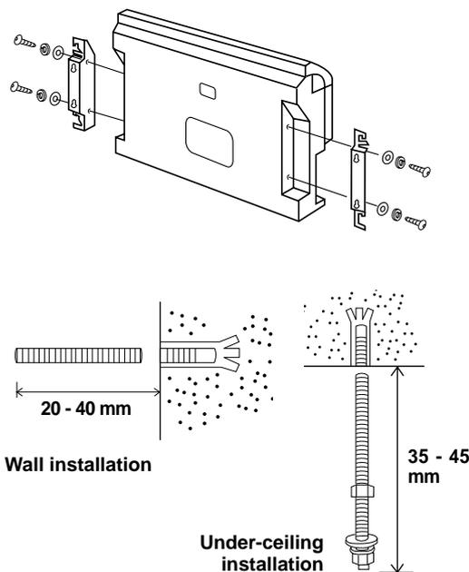
**EG KIT FOR UNDER-CEILING OR WALL INSTALLATION (ALREADY INSTALLED)**
