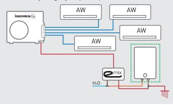
Heat pump system for underfloor heating/cooling applications with dehumidifier ducted system witch provide air distribution through small outlets. Simultaneous domestic hot water service during heating or cooling. Great solution for independent house or villas.
