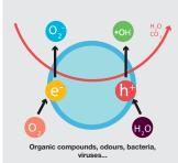
A8 is equipped with an active photocatalytic filter, which is able to significantly reduce the bacterial load in the environment thanks to the titanium dioxide oxidation process activated by completely concealed special UV LEDs that are fully compliant with EU standards. This filter uses the oxidising power of Titanium Dioxide (TiO<sub>2</sub>) to destroy bacteria and inhibit viruses. It also effectively reduces dust and dirt particles and helps to prevent unpleasant odours.
