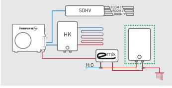
Air to water heat pump for underfloor heating/cooling applications (also in multi zones) and contemporary domestic hot water service with integrated buffer tank (eMix tank solution).
