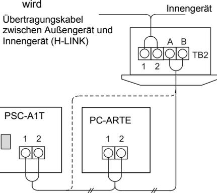
Gedrilltes 1P-0.75mm<sup>2</sup>-Kabel (max. 100m).
