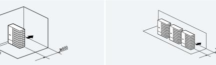
Allow 100 mm of space between units. Both right and left sides shall be open.  $% \label{eq:controller}$
