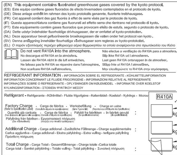
Figure 1. F-Gas Label with Protection Plastic Film
