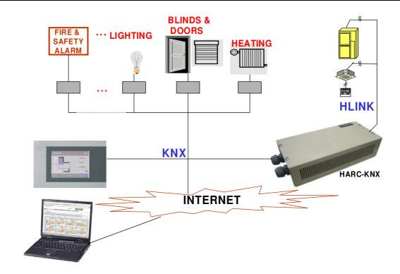
HC-A16KNX can be connected in an H-LINK 1 and/or H-LINK 2 communication line.
