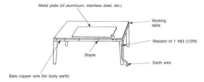
Fig. 3. Grounding of the working table
