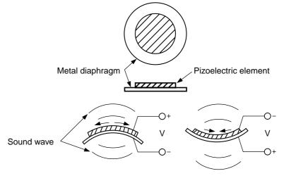
Fig. 3-2 Buzzer Operation
