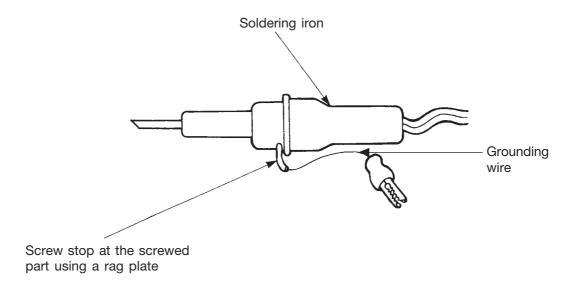
Fig. 4. Grounding a soldering iron
