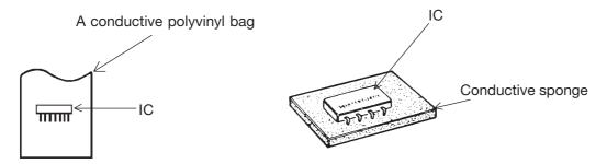
Fig. 1. Conductive Container
