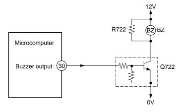
Fig. 3-1 Buzzer Circuit
