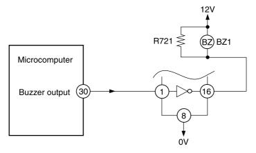
Fig. 4-1 Buzzer Circuit
