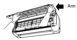
When the front panel is fully opened with both hands, push the right arm to the inside to release it, and while closing the front panel slightly, put it out forward.
