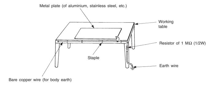
Fig. 3. Grounding of the working table
