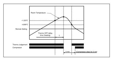
Thermo OFF delay time (heating) - preset value in EEPROM of the indoor unit.
