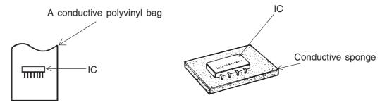
Fig. 1. Conductive Container
