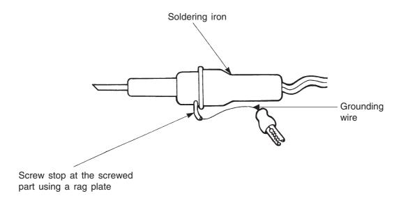
Fig. 4. Grounding a soldering iron
