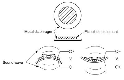
Fig. 4-2 Buzzer Operation
