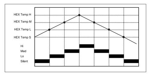
Note: Value of HEX Temp H, HEX temp M, HEX temp S are preset value in the EEPROM. As the heat exchanger sensing temperature varies, fan speed varies.
