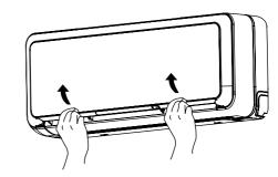
Vacuum dust from the air filter and air cleansing filter using vacuum cleaner. If there is too much dust, air filter only rinse under running tap water and gently brush it with soft bristle brush. Allow filters to dry in shade.
