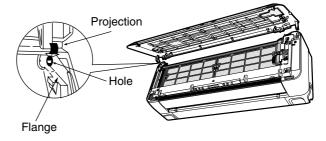
Move the projections of the left and right arms into the Flanges in the unit and securely insert them into the holes.
