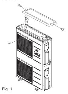
(3) Slightly widen the electric part cover to the left and right, and then lift the cover to remove it.
