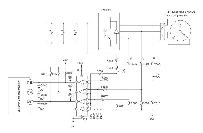
Fig. 6-1 Rotor magnetic pole position detection circuit
