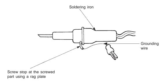
Fig. 4. Grounding a soldering iron
