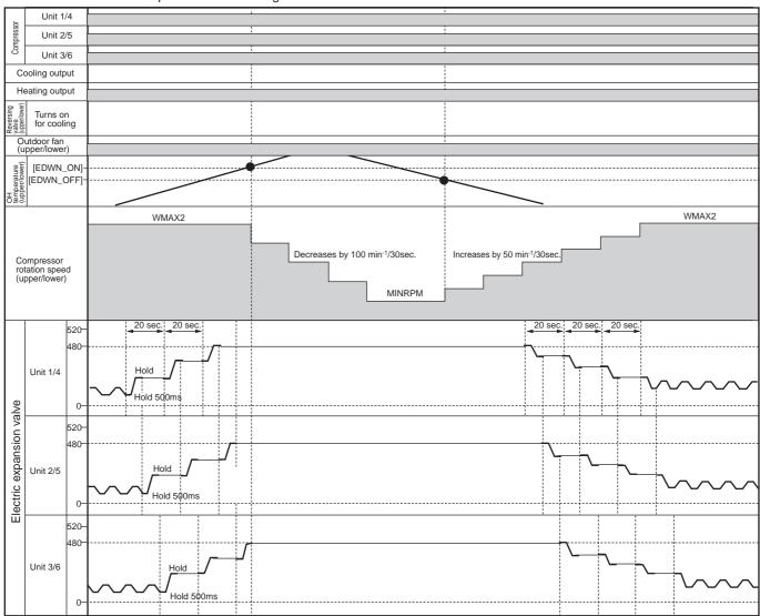
\* Operation with one unit in heating or cooling mode and with two units in cooling mode is the same as in the above diagram.
