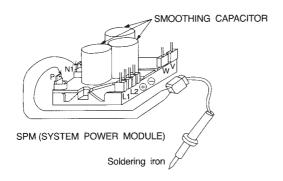
Screws of system power module are live parts: Do not touch them. Screw tightening torque and method are strictly specified. When the screw is loosened or removed once, be sure to tighten according to the procedure shown on the right, with tightening torque of  $0.8 \pm 0.2 N$  m.
