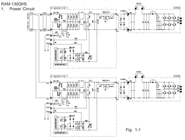
This circuit full-wave rectifies 220-240 AC applied between terminals L and N, and boosts it to a required voltage with the active module, to create a DC voltage.
