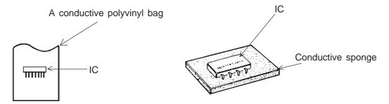
Fig. 1. Conductive Container
