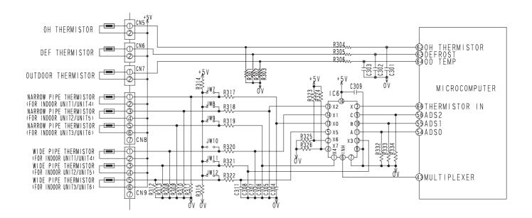
Fig. 10-1 Temperature Detection Circuit
