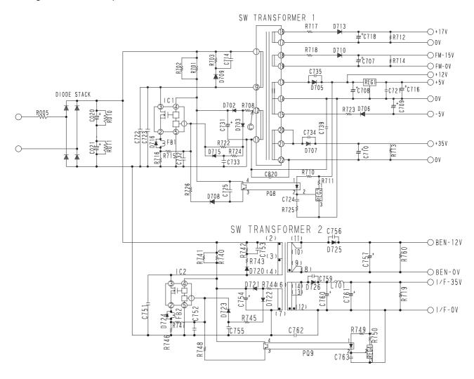
Fig. 4-1 Power circuit for P.W.B.
