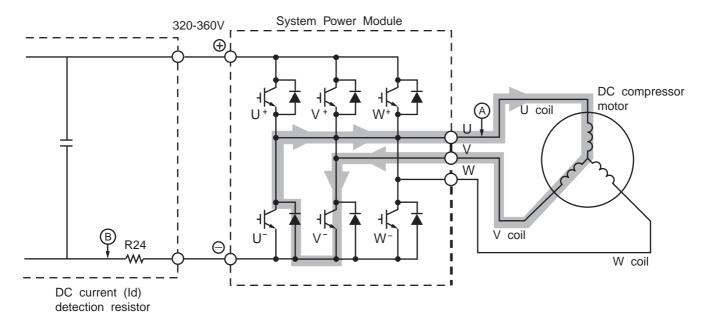
Fig. 3-4 System Power module circuit (U<sup>+</sup> is OFF, V<sup>-</sup> is ON)
