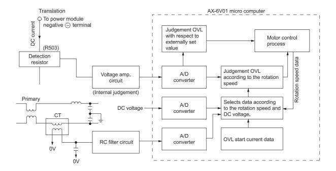
Fig. 8-1 Overload Control System Configuration
