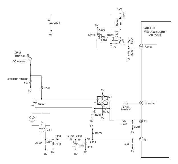
Fig. 7-1 Peripheral circuit of microcomputer (AX-6V01)
