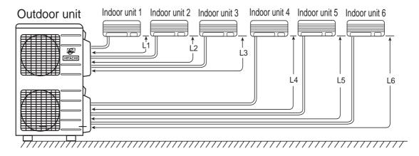
(L1 + L2 + L3) = (L4 + L5 + L6) = Maximum 45m Minimum piping length for each indoor unit is 5m. Maximum piping length for one indoor unit is 25m.
