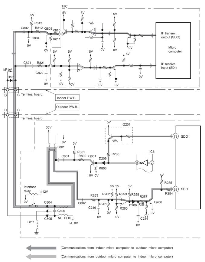
Fig. 2-1 Indoor / Outdoor interface Circuit
