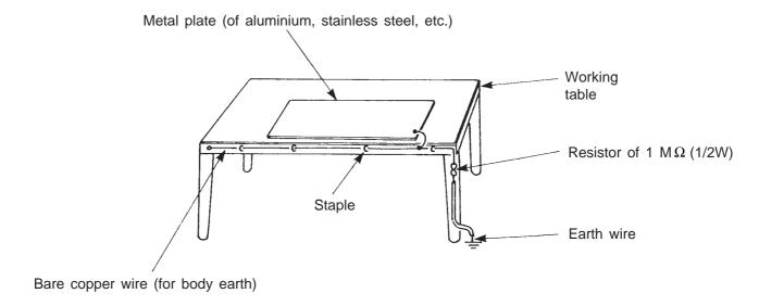
Fig. 3. Grounding of the working table
