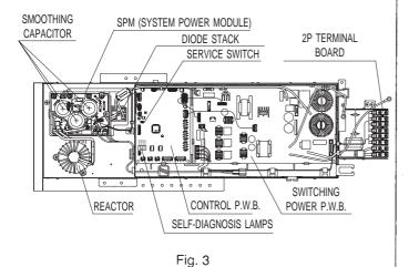
(6) When installing the electric part cover, fit the cover approximately horizontally so that it does not catch the terminal board or resin sleeve of cord.
