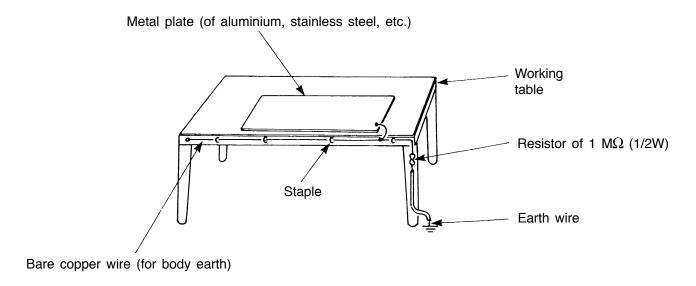
Fig. 3. Grounding of the working table
