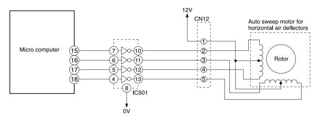
Fig. 5-1 Auto Sweep Motor Circuit (Horizontal air deflectors)
