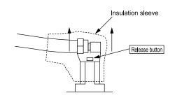
Horizontal type (with insulation sleeve) Pull out from top of insulation sleeve while pushing the release button.
