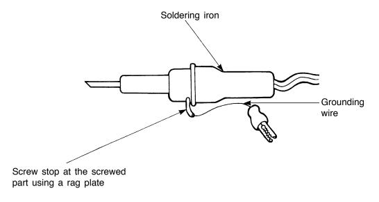
Fig. 4. Grounding a soldering iron
