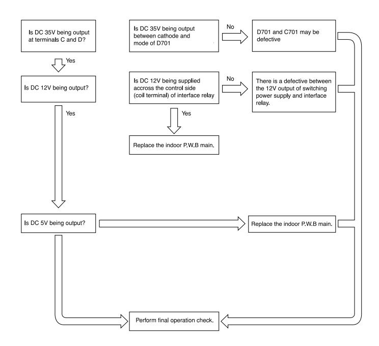
CHECKING THE OUTDOOR UNIT ELECTRICAL PART
