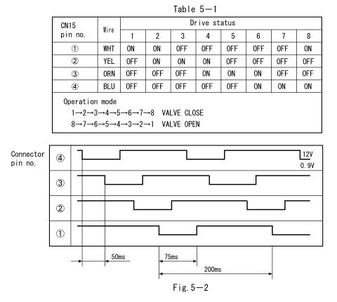
With expansion valve control, opening degree is adjusted to stabilize target temperature by detecting compressor head temperature. The period of control is about once per 20 seconds and output a few pulse.
