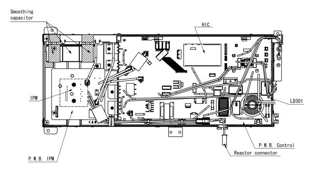
\*Be careful to avoid an electric shock as a high voltage is generated. Also take care not to cause a short-circuit through incorrect connection of test equipment terminals. The circuit board can be damage.
