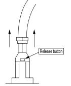
Vertical type (without casing) Pull out while pushing the release button.
