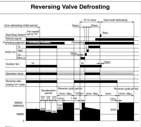
(1) The defrosting inhibit period is set as shown in the diagram below. When defrosting has finished once, the inhibit period is newly set, based on the outdoor temperature when the compressor was started. During this period, the defrost signal is not accepted.
