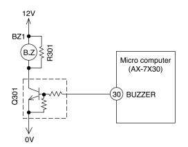
When the buzzer is to be activated, buzzer output pin (30) of the micro computer alternates between ON and OFF repeatedly at 4kHz and Q301 is turned ON/OFF accordingly. A 4kHz voltage is applied to the buzzer and the diaphragm of the buzzer vibrates to output 4kHz sound.
