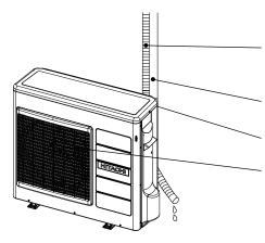
DRAIN PIPE Condensed water drain to outside.
