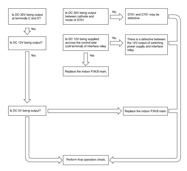
CHECKING THE OUTDOOR UNIT ELECTRICAL PART
