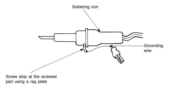
Fig. 4. Grounding a soldering iron
