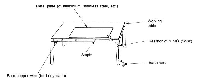
Fig. 3. Grounding of the working table
