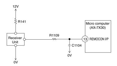
Infrared signals from the wireless remote controller are received by the light receiving unit and output after being amplified and shaped.
