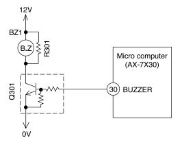
When the buzzer is to be activated, buzzer output pin (30) of the micro computer alternates between ON and OFF repeatedly at 4kHz and Q301 is turned ON/OFF accordingly. A 4kHz voltage/frequency is applied to the buzzer and the diaphragm of the buzzer vibrates to output 4kHz sound.
