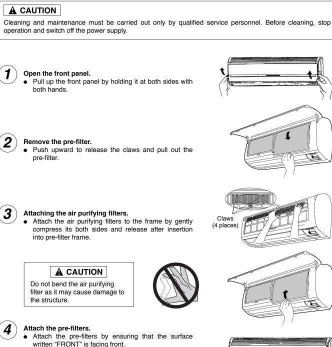
• After attaching the pre-filters, push the front panel at three arrow portion as shown in figure and close it.
