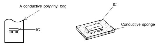
Fig. 1. Conductive Container
