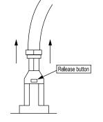
Vertical type (without casing) Pull out while pushing the release button.
