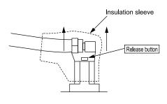
Horizontal type (with insulation sleeve)
