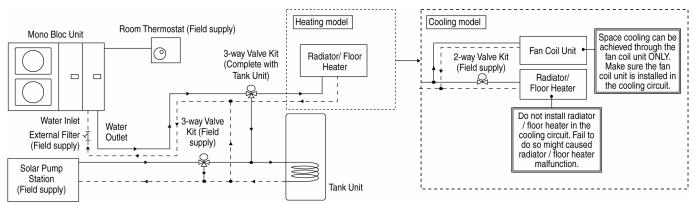
Diagram 3.1: Typical Water Piping Installation
