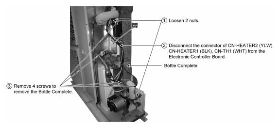
⚠ When reinstall the water pipe, use grease or water at the joining.
