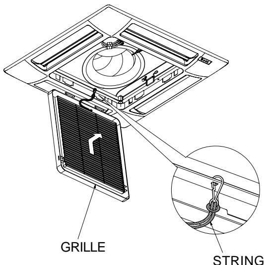
1. Detach the safety string from the frame (remember to attach it again after cleaning or maintenance).
