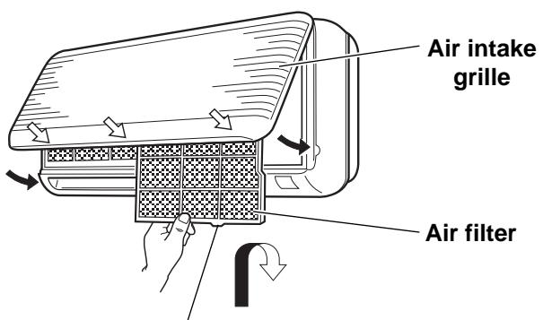
**Insert into the groove on the unit**
